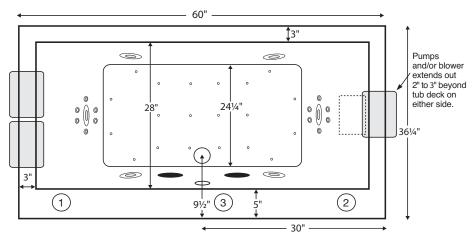
Numbered areas on tub deck represent possible locations to install cleaning systems, faucets and other fixtures. Pump and / or blower extends out 2" - 3" beyond tub deck on either side.
