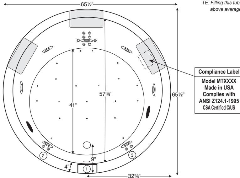
Numbered areas on tub deck represent possible locations to install cleaning systems, faucets and other fixtures. When ordering Fill-Flush and location 1 is chosen, the detergent feeder will need to be offset to the left or the right.
