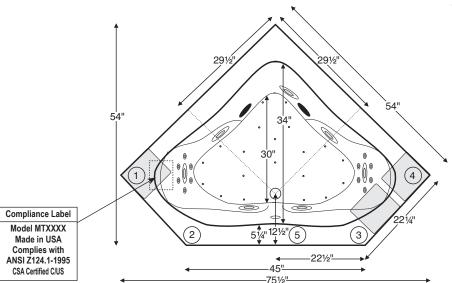
Numbered areas on tub deck represent possible locations to install cleaning systems, faucets and other fixtures.
