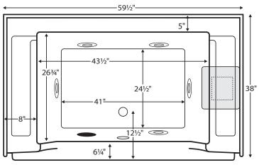
NOTE: Pump and fixtures come standard on the right. Left-hand placement is available by special request.
